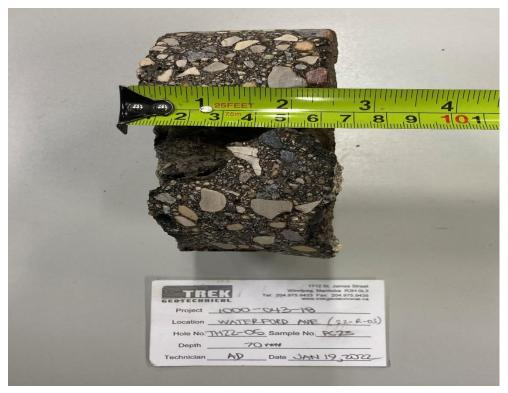
Photo 5: Pavement Core Sample at Test Hole TH22-05
