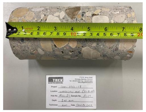
Photo 7: Pavement Core Sample at PC22-27
