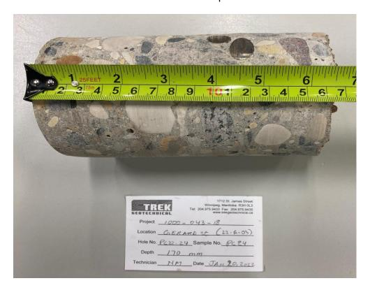
Photo 2: Pavement Core Sample at PC22-24
