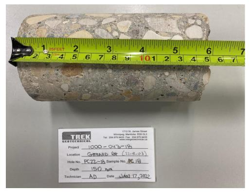
Photo 1: Pavement Core Sample at PC22-18
