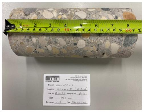
Photo 3: Pavement Core Sample at PC22-25
