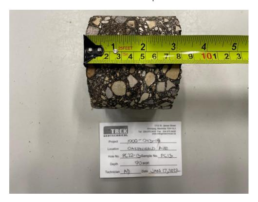
Photo 4: Pavement Core Sample at PC22-13
