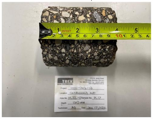
Photo 8: Pavement Core Sample at PC22-17
