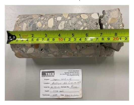
Photo 2: Pavement Core Sample at PC22-02
