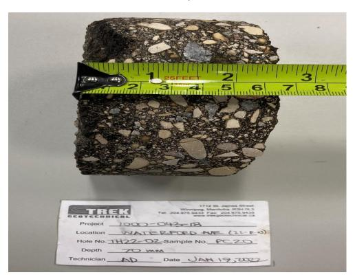
Photo 2: Pavement Core Sample at Test Hole TH22-02
