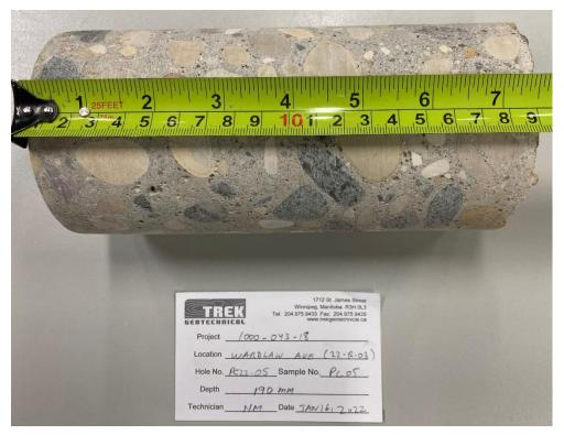
Photo 1: Pavement Core Sample at PC22-05
