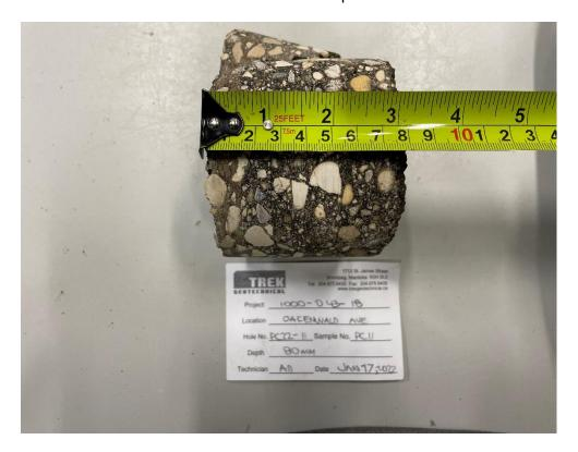
Photo 2: Pavement Core Sample at PC22-11
