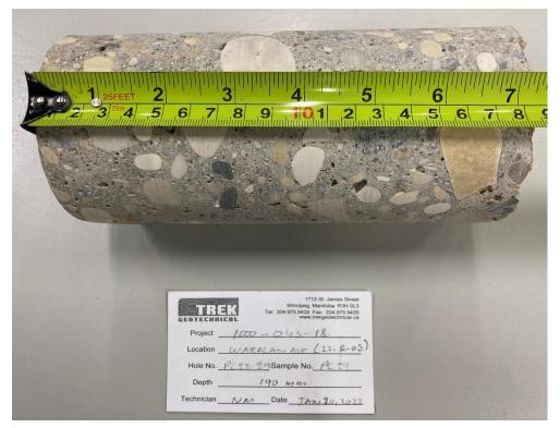
Photo 9: Pavement Core Sample at PC22-29
